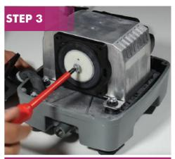
Remove the screw along with the diaphragm electrostatic membrane and depressor, diaphragm. Repeat on the opposite end of the pump.
