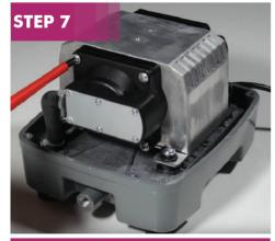
Put chamber cover back and screw four screws in. Repeat this process on the opposite side of the pump.
