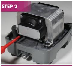
chamber cover at one end of the pump. Separate the chamber cover at the seam to expose the screw holding the white round plastic diaphragm depressor in place.
